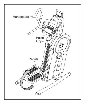
To dismount the trainer, wait until the pedals come to a complete stop. **Note: The trainer does not have a free wheel; the pedals will continue to move until the flywheel stops.** When the pedals are stationary, step off the higher pedal first. Then, step off the lower pedal.
