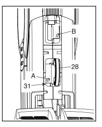
Stand on the trainer and pedal for a few moments. If the pedals still slip, step off the trainer and locate the upper Adjustment Screw (B). Tighten the upper Adjustment Screw two turns; this will tighten the Small Drive Belt (28).
