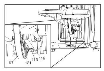
Then, plug in the power adapter and turn the Large Pulley (21) for a moment. Repeat these actions, if necessary, until the console displays correct feedback. Then, reattach the lower rear shield cover.
