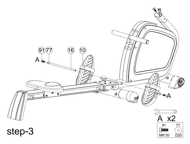
Assemble the foot pedal (10) using the axle (16), flat washer (77) and bolt (91).
