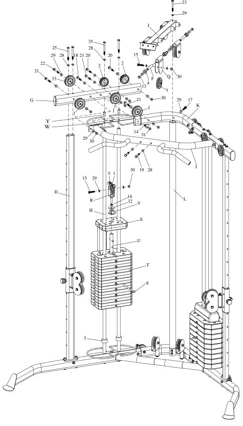
7. Slide rubber donut (3) onto guide rod (H).
