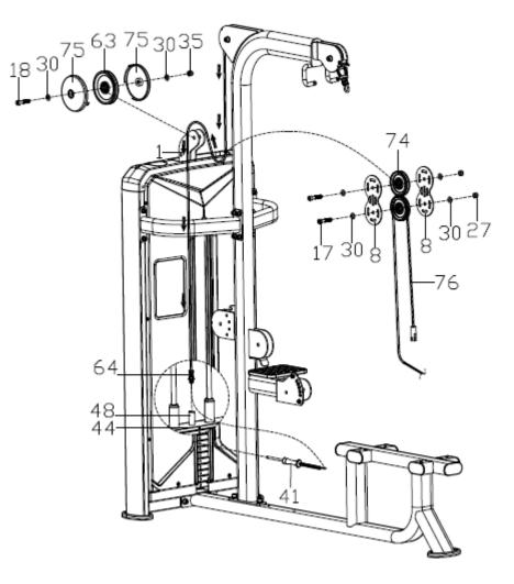
Attach the cable (76) to the frame (3) using the bolt (12), washers (31) and nut (28).
