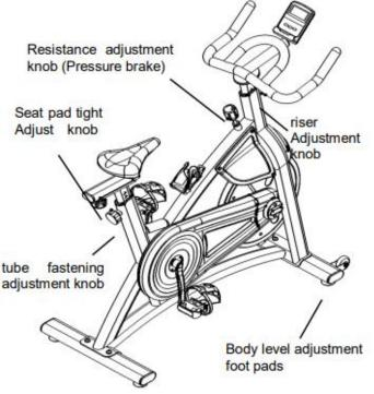
Check the fastening of all parts and adjust the desired height and position of the seat.
