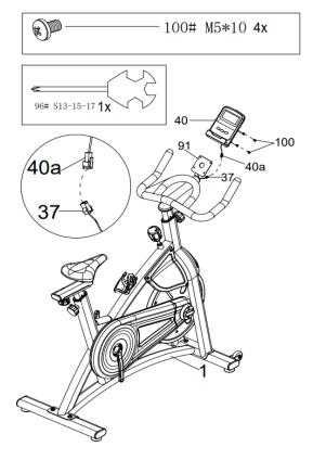
Attach the console (40) to the console holder (91) with 2x M5\*10 screws (100)
