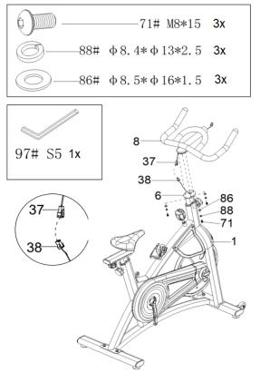
Connect the sensor cable from the handles (37) to the cable leading from the main frame (38). and then fix with 3x M8\*15 screws, 3x  $\varphi 8.5*13*2.5$  spring washers (88) and 3x  $\varphi 8.5*16*1.5$  flat washers (86).
