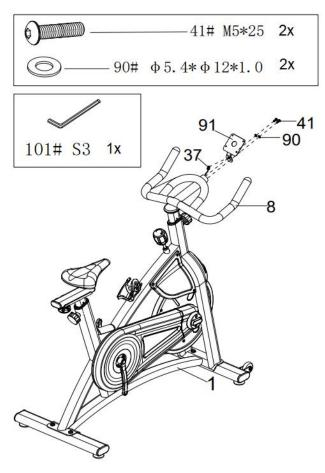
Pass the sensor cable (37) through the console holder (91), then attach the console holder (91) to the handles (8) with 2x M5\*25 screws (41) and 2x  $\varphi$ 5.2\*12\*1.0 washers (90)
