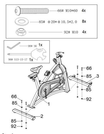
Attach the front stabilizer (3) and rear stabilizer (2) to the main frame (1) with 4x M10\*60 screws (66),  $8x \notin 10.5*20*2.0$  flat washers (85), and 4x M10 nuts (92).
