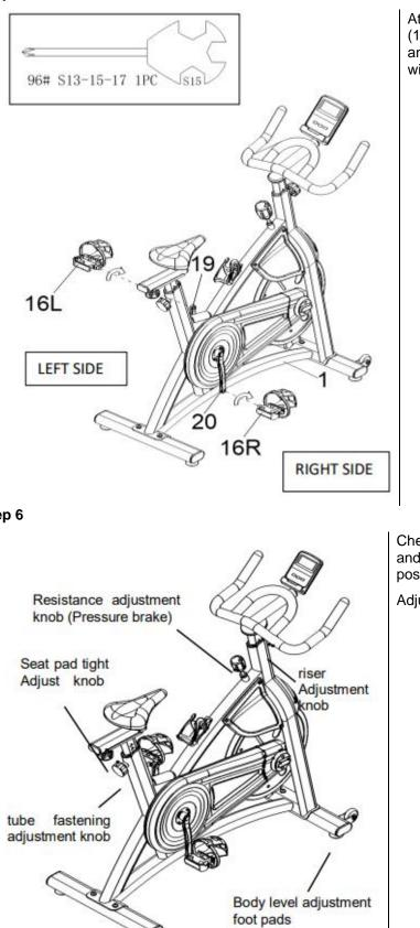
Attach the right (16R) and left (16L) pedals to the right (20) and left (19) cranks. Tighten with wrench (96)
