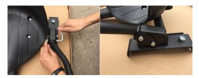
4. Assembly the front tube: please put the tube into it, and adjust the suitable hole.
