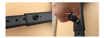
5.Put the whole hover kart to the scooter:Adjust the nut on the shelf to fit the size of hover board. Assembly the hover kart on the scooter with the bandage, please check the bandage is firm before using the hover kart.
