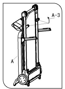
Turn the Part A-3 according to the direction of the arrow.
