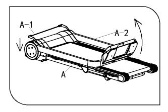
Press down the part (A-1) and then pull up the Left & Right part (A-2) as the direction of the arrow.
