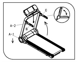
Put the Main Frame A on the ground and press down the part A-1, then pull up the part A-2 till you hear the sound "KA". At the end, turn the Handle Bars (B & C) down with clockwise rotation.
