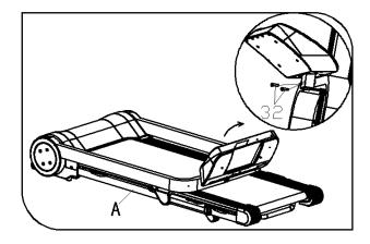
Pull up the console as the direction of the arrow. Please make sure the connect wires of console is not pressed. Lock the (#32) screw with #5 wrench.
