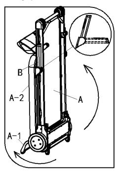
Turn the handle bars up and put them on the position shown on the picture. Hold the A-1, turn the part A-2 down to the Main Frame till you hear the sound "KA". Then, fold the running deck as the direction of the arrow up to the position shown in the picture.
