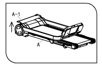
Pull up the part (A-1) as the direction of the arrow. And put the main frame (A) on vertical direction.
