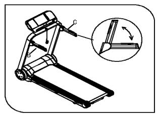
Turn the handle bars (B & C) down with clockwise rotation.
