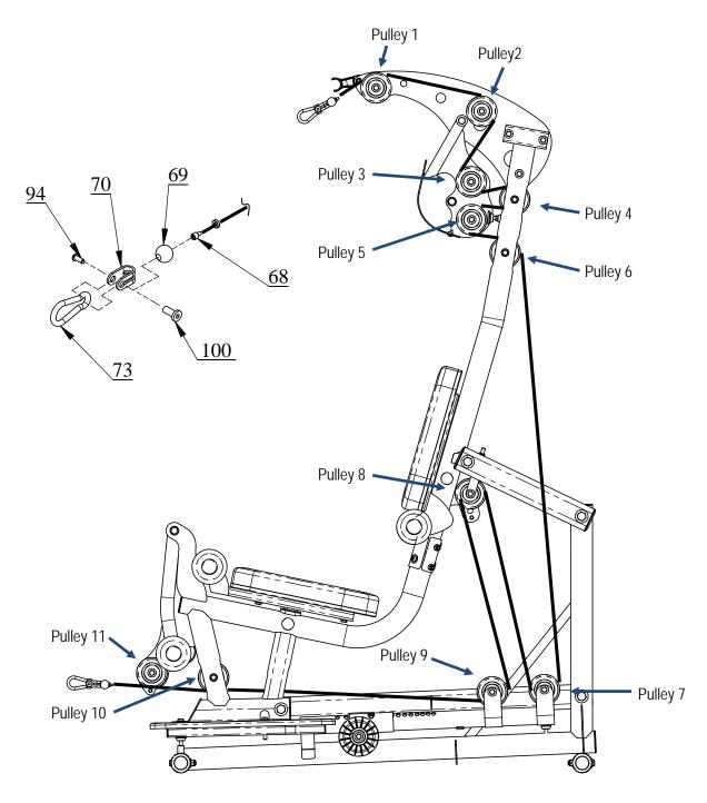
Began at the top of the machine and run the cable sequentially from pulley #1 to pulley #11, as shown in the above drawing. Once complete, finish both cable ends with a plastic ball (#69), "U" bracket (#70), flat head nut (#100), button head bolt (#94), and a spring clip (#73). Look back over the cable routing to make sure that the cable is sitting securely in each pulley.
