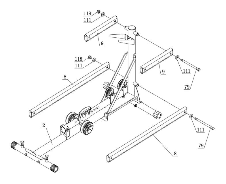
Attach Lower Arms (#8) to Base Frame Assembly (#2) using: One (M16x230 Hex Bolt)
