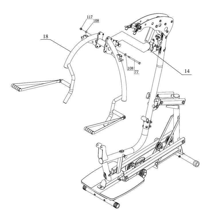
Attach Press Arm (#18) to Press Arm Mount (#14) using: One (M12\*160 Hex Bolt)
