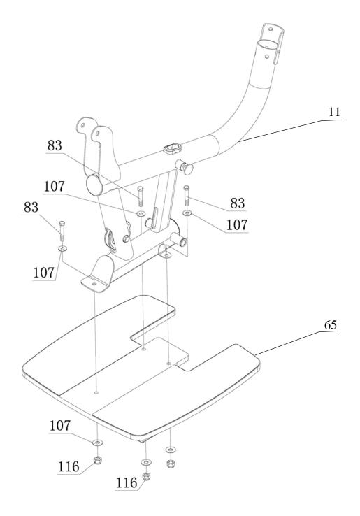
Attach Lower Main Frame (#11) to Foot Plate (#65) using: Three (M10x60 Hex Bolt)
