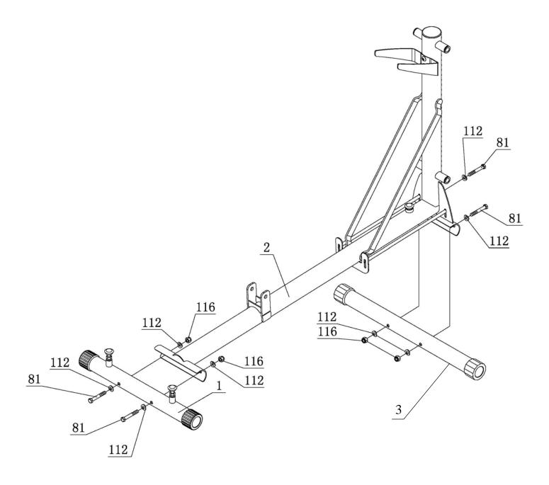
Attach Front Foot Assembly (#1) to Base Frame Assembly (#2) using: Two (M10x70 Bolts)
