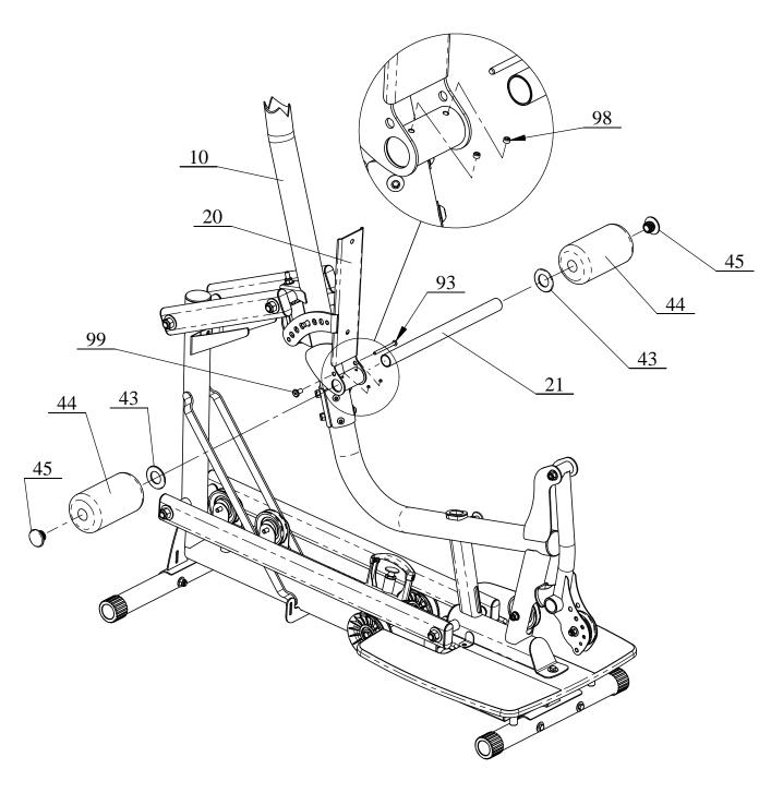
Attach Back Pad Tilt Frame (#20) to Upper Main Frame (#10) using:
