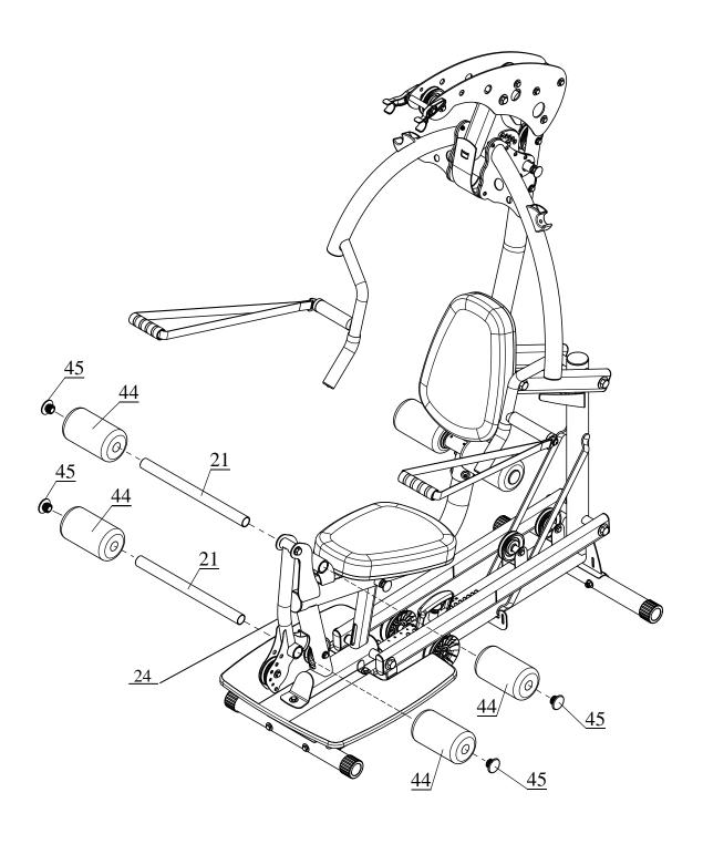
Attach 4 Foam Rollers (#44) to Leg Extension Assembly (#24) & Seat Stem (#23) using:
