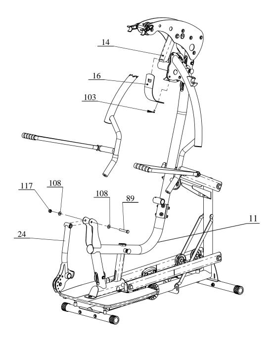
Attach Leg Extension Assembly (#24) to Lower Main Frame (#11) using:
