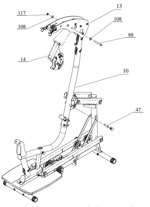
Attach Press Arm Mount (#14) to Top Beam Plates (#13) using: One (M12\*100 Hex Bolt)
