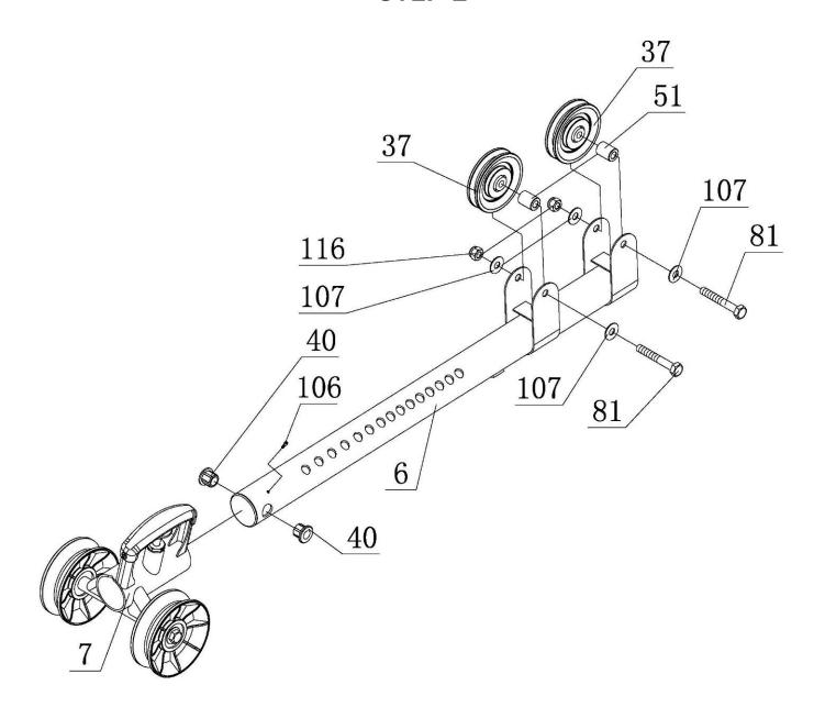
Attach Slider Assembly (#7) to Weight Selector Tube(#6).
