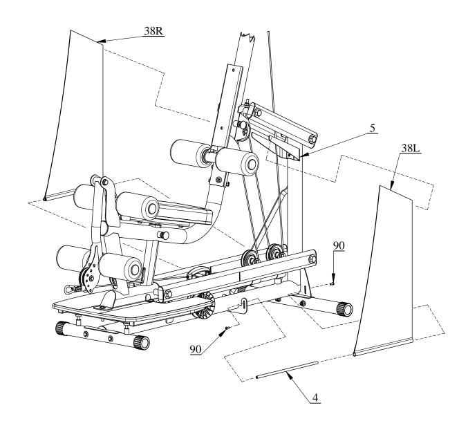
Attach Left and Right Shrouds (#38L & #38R) by first slipping the top of each Shroud onto the horns of the upper shroud mount (#5), as shown above. Make sure seams are to the inside. Next, slide rods (#4) into the bottom of each shroud and attach to frame using:
