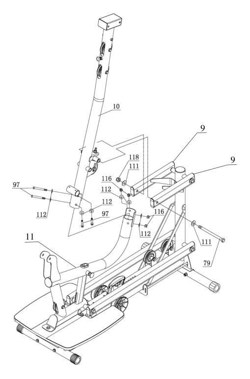
Attach Upper Main Frame (#10) to Lower Main Frame (#11) using:
