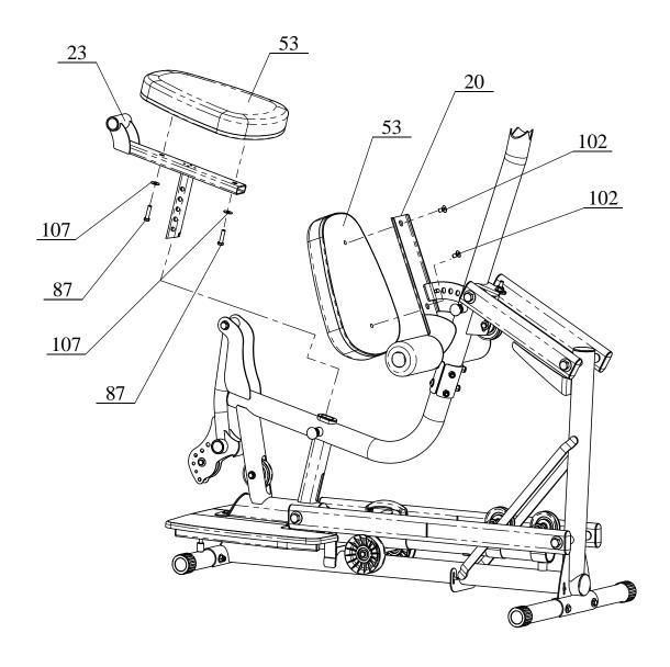
Attach Seat Pad (#53) to Seat Stem (#23) using: **Two (M10\*40 Hex Bolts) Wrench Tighten Now**.
