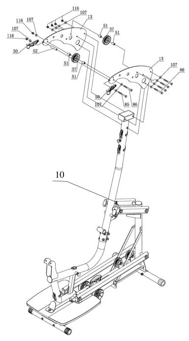
Attach Top Beam Plates (#13) and One 3 ½" Pulley (#37) to Upper Main Frame (#10) using:
