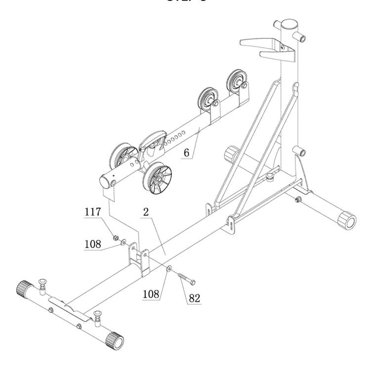
Attach Weight Selector Tube (#6) to Base Frame Assembly (#2) using:
