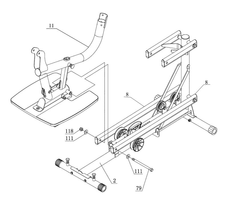
Attach Lower Main Frame (#11) to Lower Arms (#8) using: One (M16x230 Hex Bolt)
