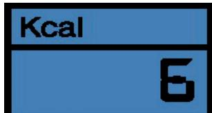
Shows the energy consumption, based on a efficiency of 22% to provide the mechanical power. Range from 10-9990Kcal.
