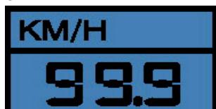
Display of speed in km/h, 0-99.99km/h, (theoretical assumed value), which cannot be compared with the speed value of a regular outdoor bike.
